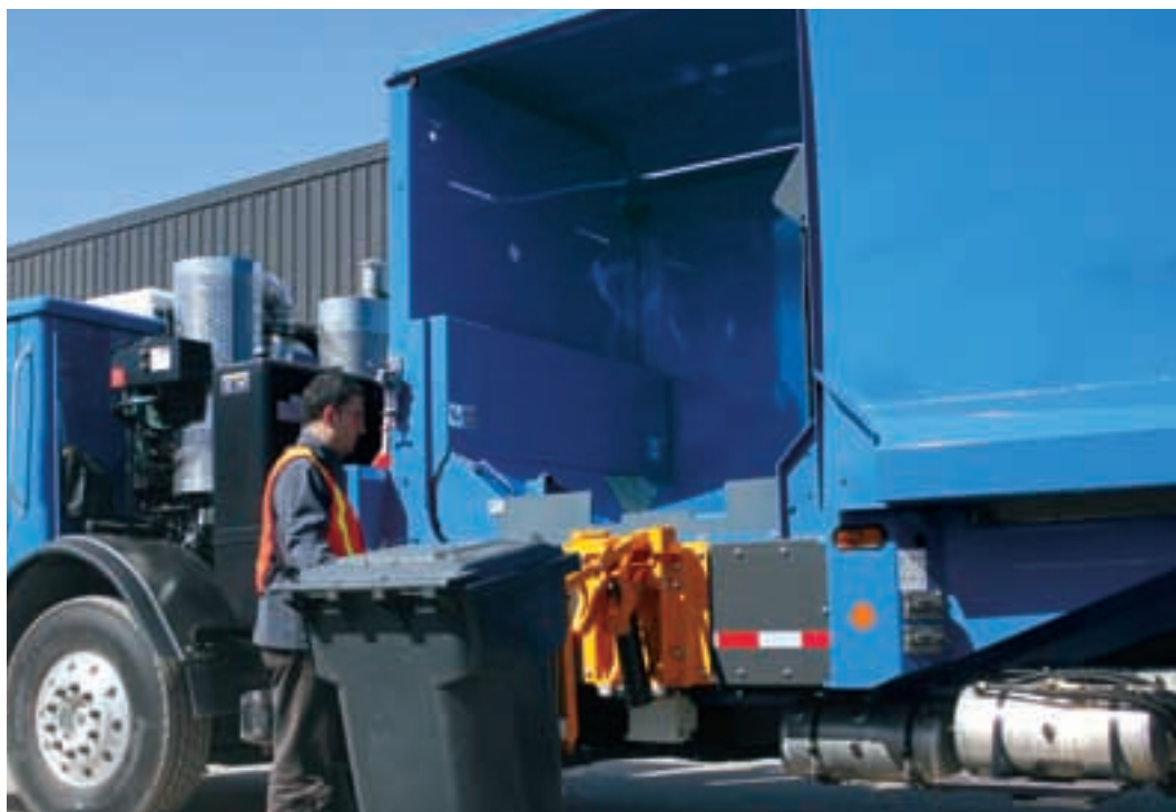
Semi-automated cart tipper on street side
