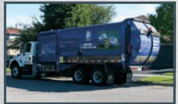
60/40, 40/60, 70/30, 30/70, 15/85 or 50/50 split bodies with single or split chute inside the hopper
