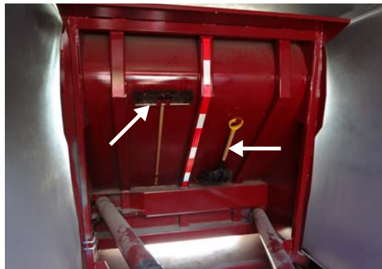
Figure 4-9 Cleaning tools behind the packer
