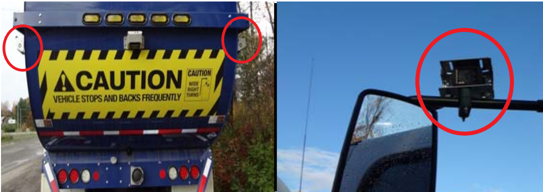
Figure 2-15 Cameras on both sides of the tailgate (left) and on the left-hand side mirror (right)
