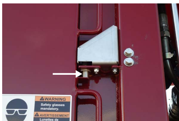
Figure 2-16 Side Access Door proximity switch
