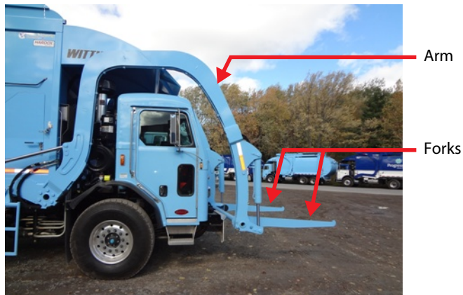
Figure 4-3 Lifting arms and forks
