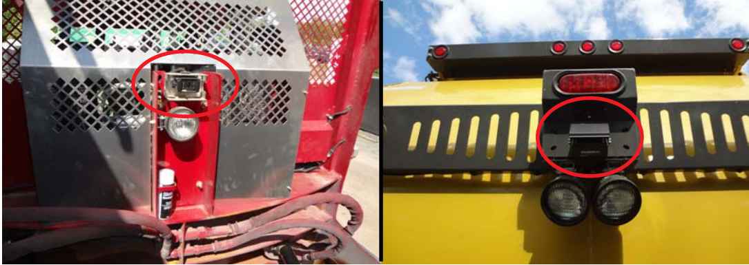
Figure 2-15 Cameras on both sides of the tailgate (left) and on the left-hand side mirror (right)
