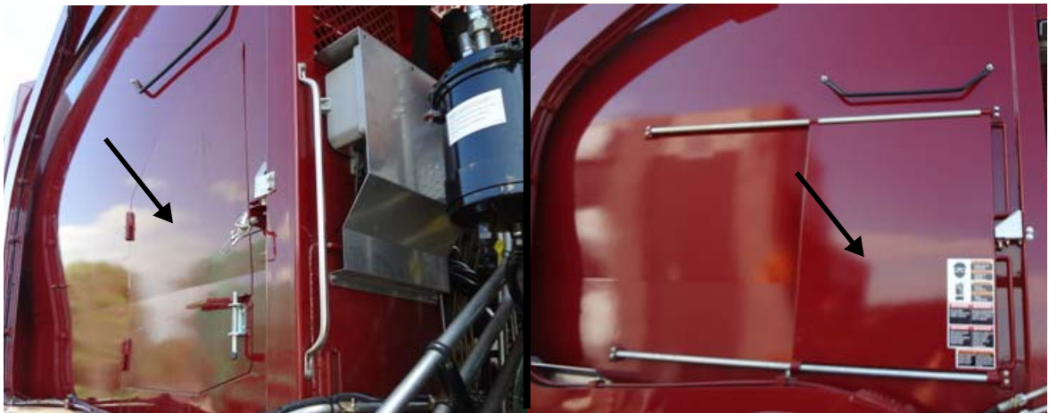
Figure 4-1 Hinged side access door (left); Sliding side access door (right)
