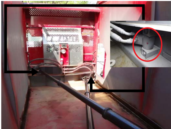
Figure 2-3 Standard manual grease fittings (front-end cylinder pins)
