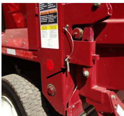
Figure 2-12 Tailgate safety pin in locking position
