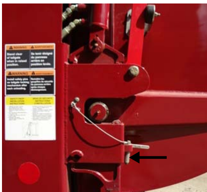
Figure 2-13 Tailgate safety pin in storage position
