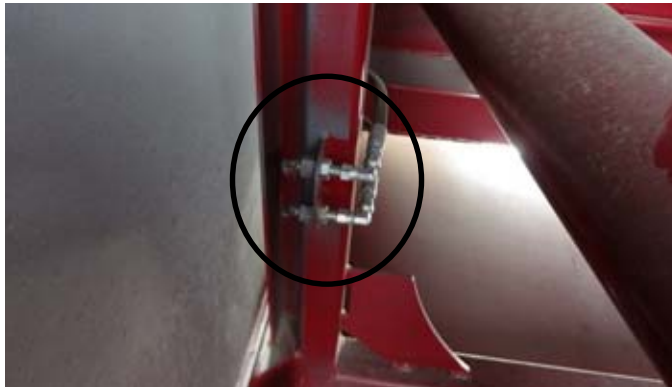
Figure 2-2 Standard grease fittings on back of packer blade
