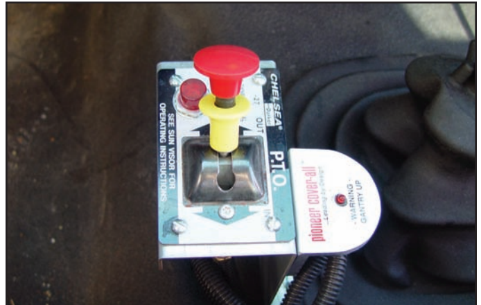
2. Put the truck in neutral and engage the PTO. Run RPM as needed.
