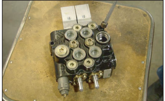
2. Install a 3/8" straight thread pipe plug into lower portion of cavity to activate the power beyond feature. Use thread sealer (tape sealers not recommended).
