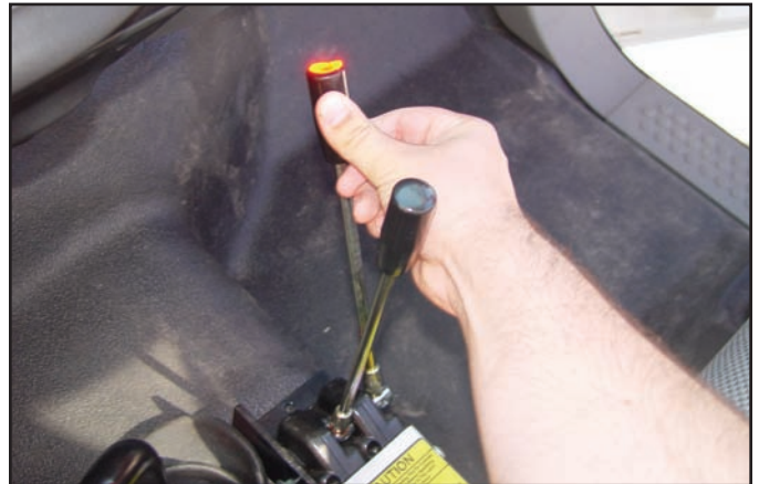
2. Push the red (lift) lever until the boom bottoms out. Keep pushing the lever forward until steps 3-5 are complete.
