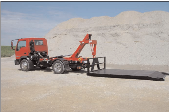
1. Position the truck in line with the body you intend to pick up.
