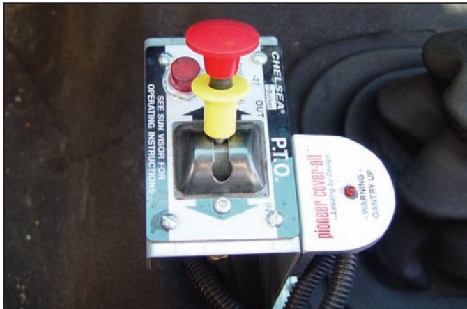
1. Engage the PTO. Run the truck at 1300 RPM.
