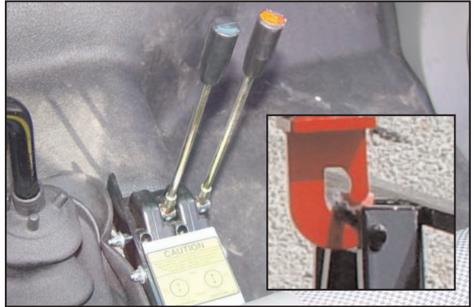
2. Engage the hook to the body by maneuvering the hooklift with the red(lift) lever. Run RPM as needed.
