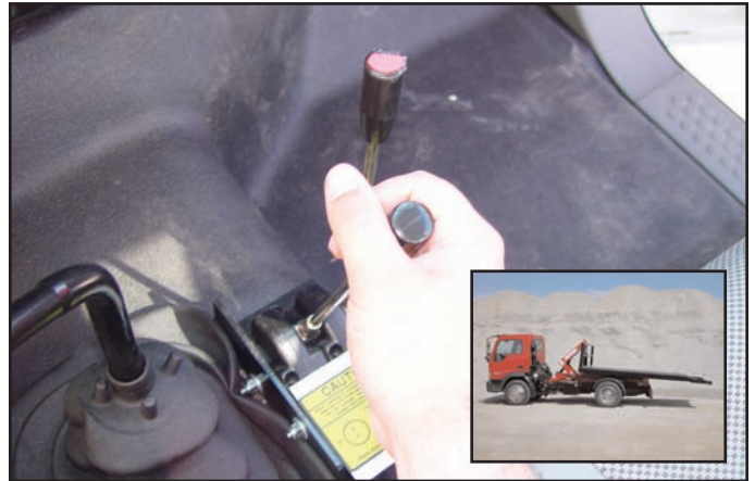
4. Pull the tilt lever until the cylinder is fully extended, thus releasing tabs.
