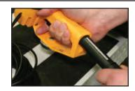
3. Attach the other end of the back-up cord to the connector currently used by the antenna on the control receiver. The control receiver is located on the back of the crane mast.
