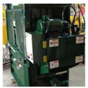
The side-mounted, self-contained power unit is convenient for maintenance and servicing.
