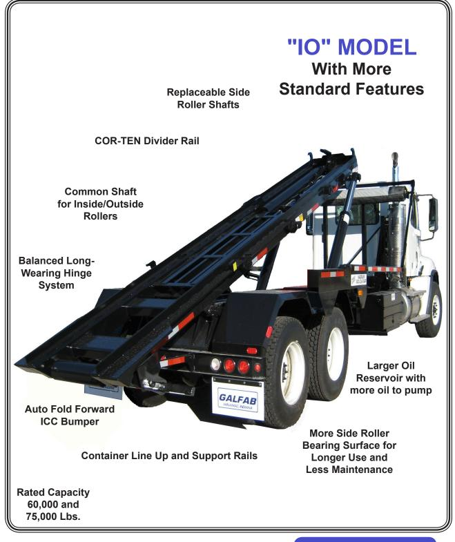
GALFAB roll-off hoists are designed and built with the user in mind. GALFAB's hoist is jig-built for quality, accuracy, and consistency. GALFAB's auto fold forward DOT bumper folds toward the truck.
