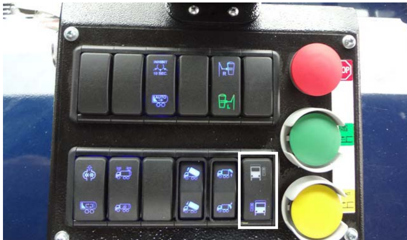
Figure 7-5 Packer control selector switch
