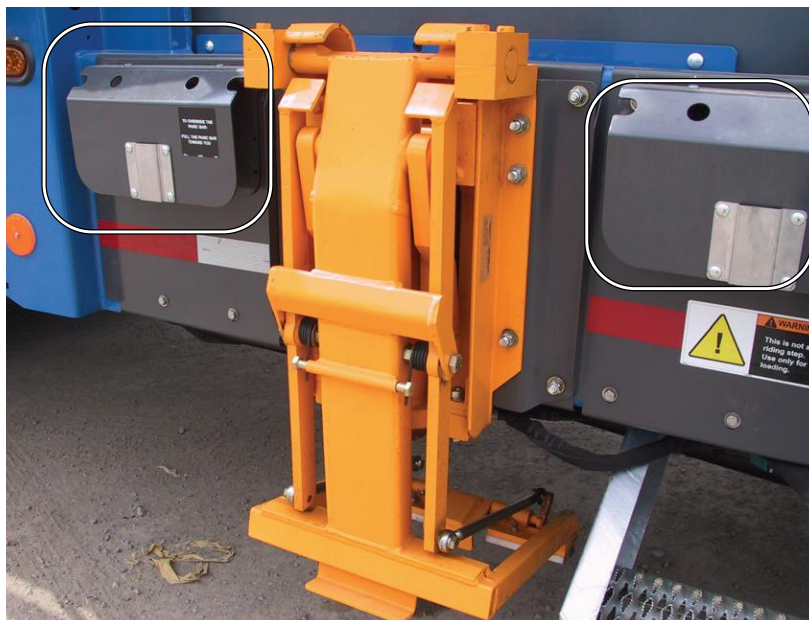
Figure 2-2 Panic bar on each side of a cart tipper
