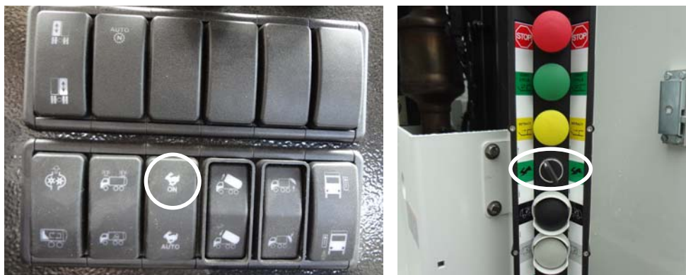
Figure 7-4 Speed-up switch/button: on the console panel (left); on the control station (right)
