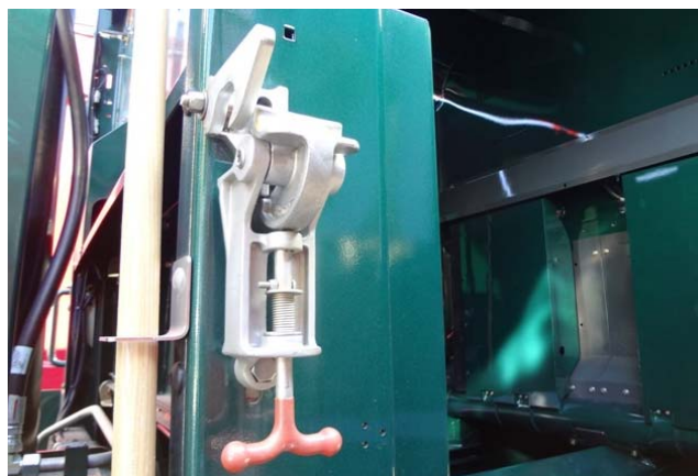
Figure 2-5 Standard door lock when no arm or Dutch door is installed
