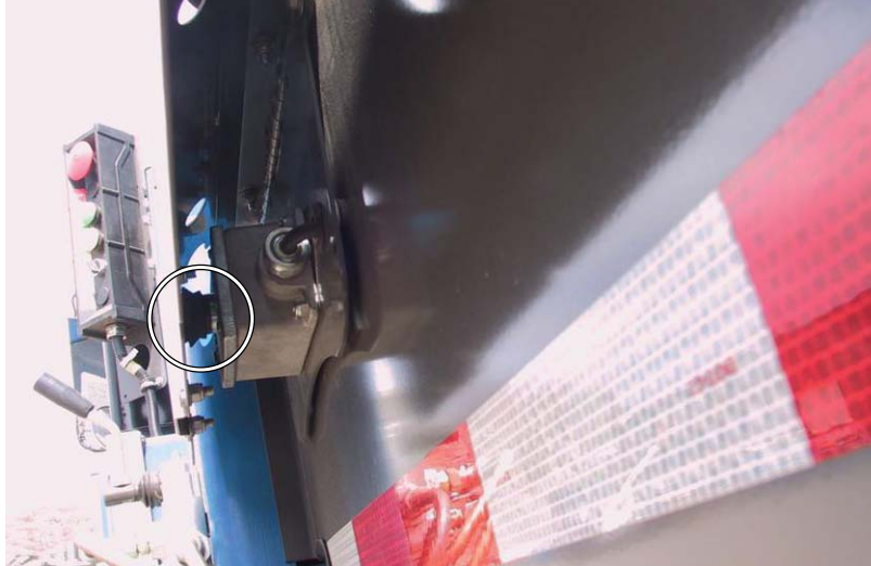
Figure 2-4 Emergency stop button underneath the panic bar
