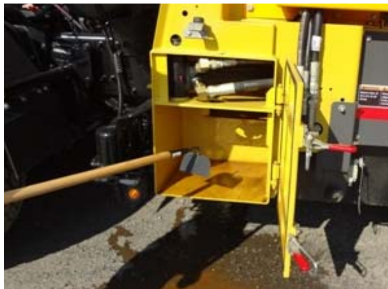
Figure 10-7 Clean-out trap door
