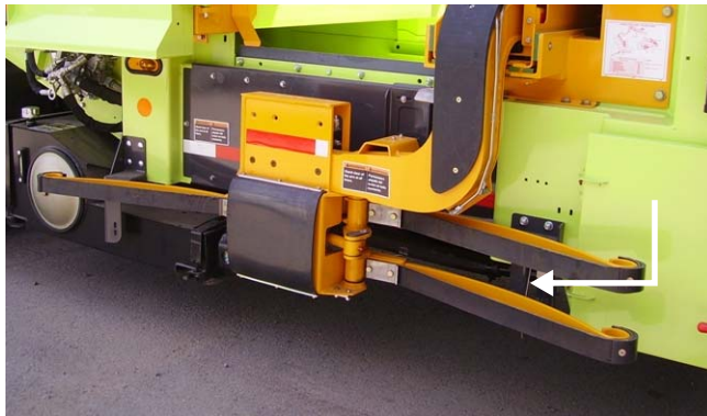
Figure 4-5 Mid-height limit switch (left), parked limit switch (right)
