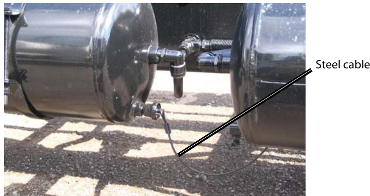
Figure 10-5 Air tank with steel cable on drain valve
