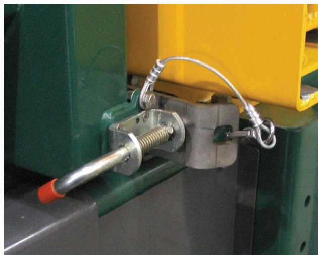
Figure 2-6 Door lock on vehicles equipped with Helping Hand™ and Dutch door options
