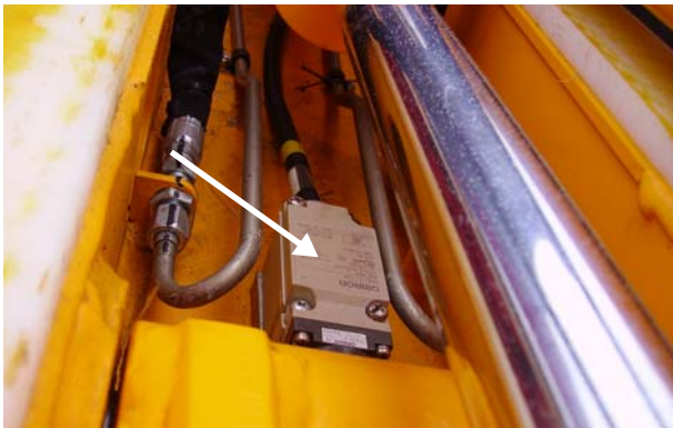
Figure 4-5 Mid-height limit switch (left), parked limit switch (right)
