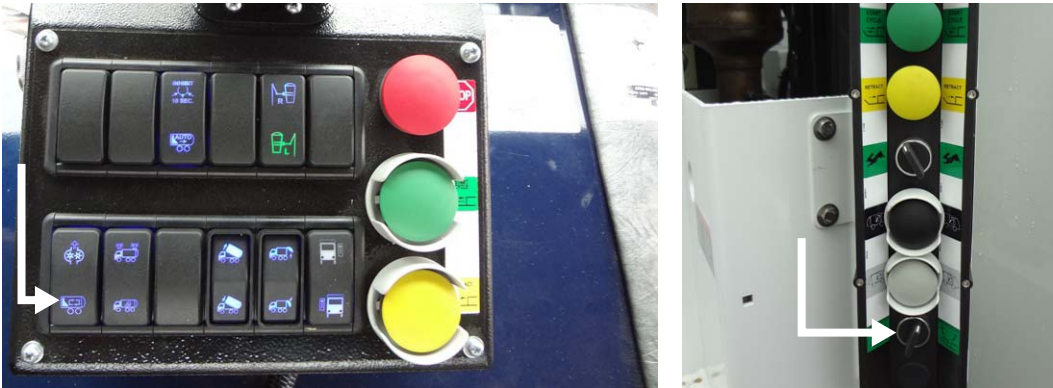
Figure 7-10 Multicycle control switch: on the in-cab control panel (left), on the packer control station (right)
