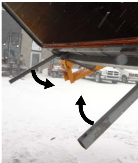
Figure 2-6 Putting back props into stored position
