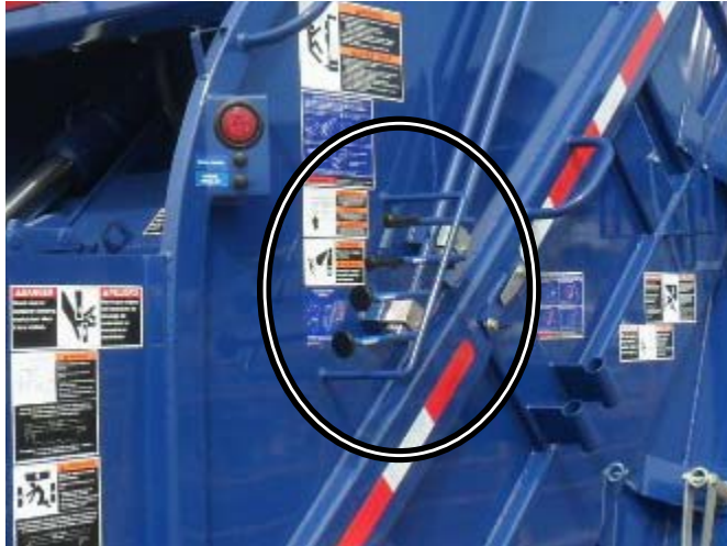
Figure 1-6 Operating controls (packer, carrier panel, container handling system)
