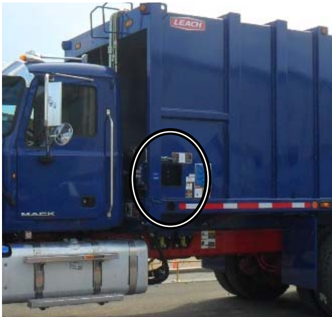
Figure 1-7 Pushout panel and tailgate operating controls
