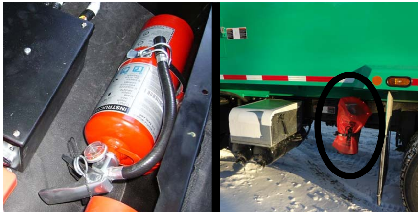
Figure 2-1 5-lb fire extinguisher (left); optional 20-lb fire extinguisher (right)
