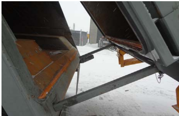
Figure 2-5 Props leaned against body base
