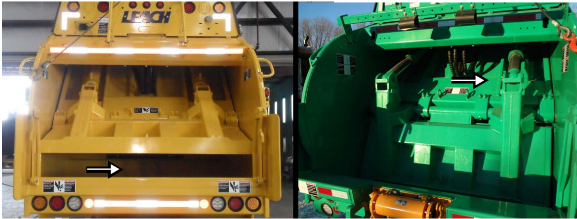
Figure 1-3 Hopper (left); Carrier panel (right)
