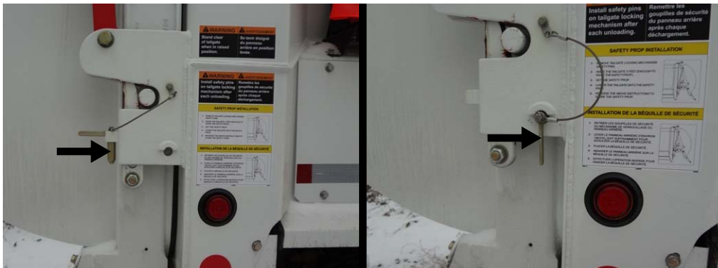
Figure 2-10 Safety pin (in storage position, left; in locking position, right)
