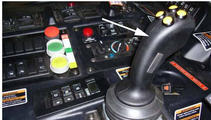
Figure 9-20 CAN bus-based multiplex joystick
