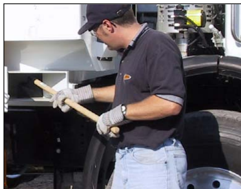
Figure 3-6 Removing debris through the clean-out trap
