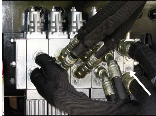
Figure 5-23 Main relief valve adjustment screw
