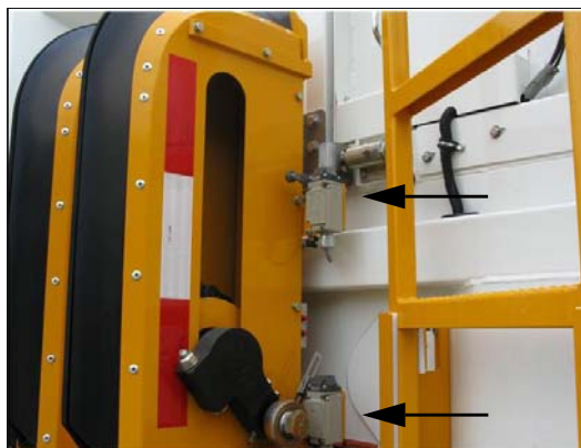
Figure 10-7 Auto-closing limit switch (lower) and camera switching limit switch
