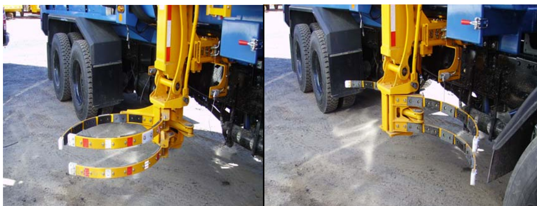
Figure 10-8 Gripper closed (left) and open (right)
