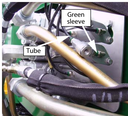
Figure 8-6 Removing the air tube from the actuator
