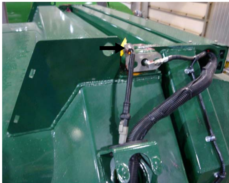
Figure 3-89 Tailgate fully open proximity switch
