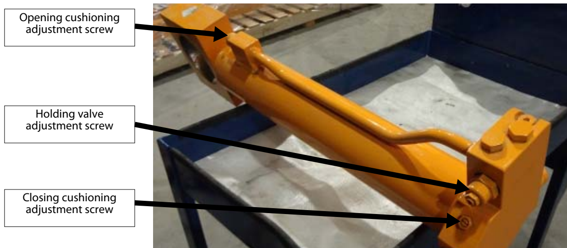
Figure 10-20 Holding valve adjustment screw (up/down cylinder) - HD arm
