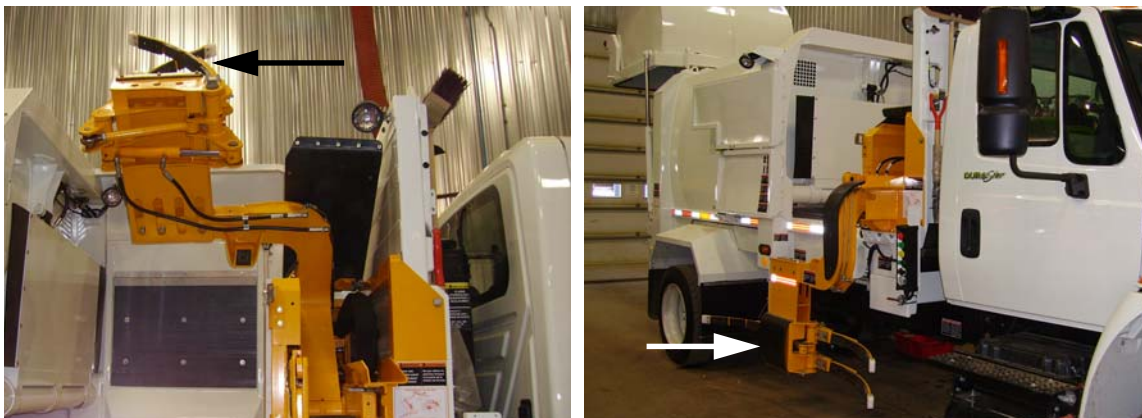
Figure 10-7 Gripper closed (left) and open (right)
