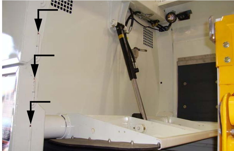
Figure 4-20 Grease fitting on top of door hinges
