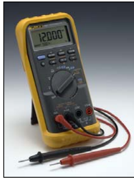
Figure 8-1 Digital Multimeter or VOM (Volt-Ohm-Milliammeter)
