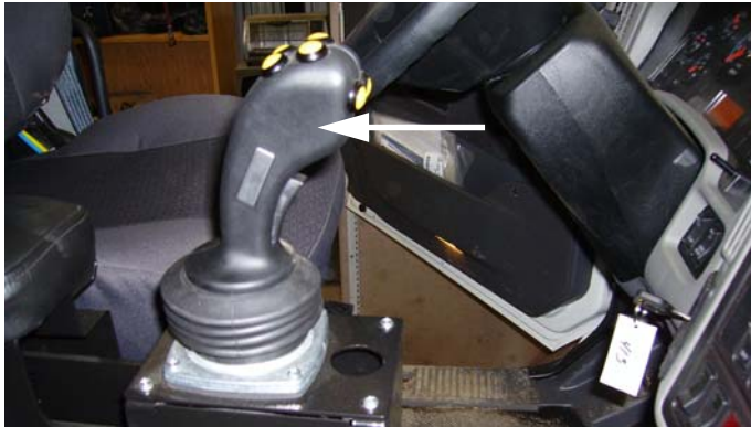
Figure 9-21 CAN bus-based multiplexed system joystick
