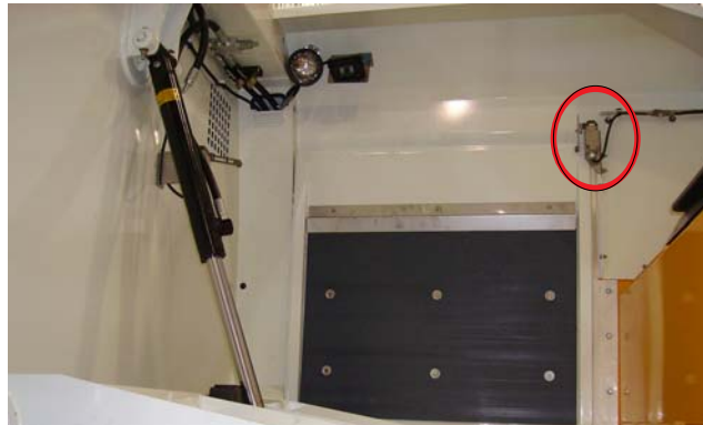
Figure 3-29 LHS hopper door limit switch
