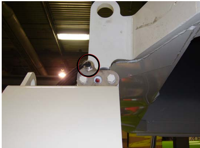
Figure 3-28 Tailgate fully open proximity switch
