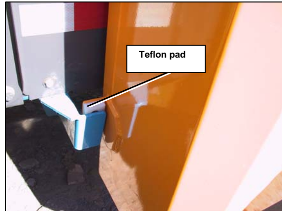
Figure 137. Small teflon pad located on the L-H side of the glass compartment
