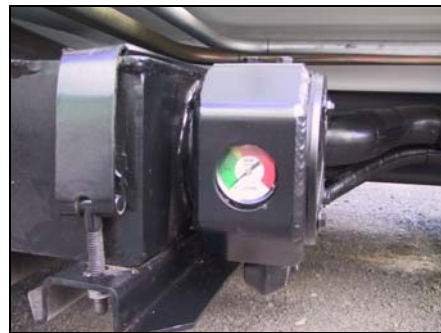
Figure 103. Filter restriction indicator
