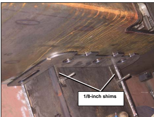
Figure 63. Shims below the scraper
