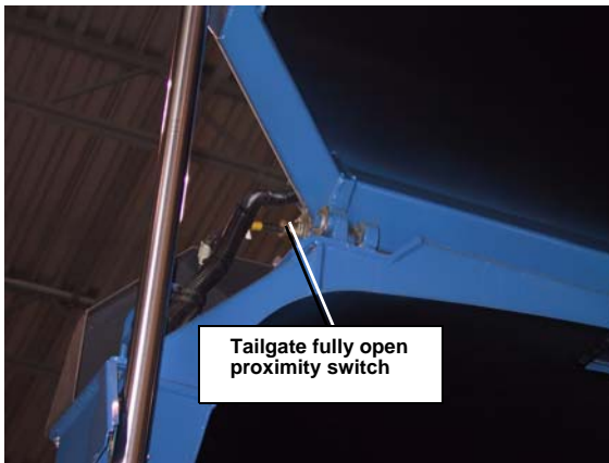
Figure 93. Tailgate fully open proximity switch (optional)
