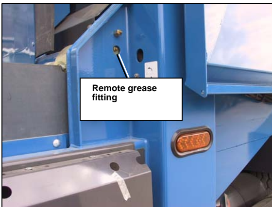
Figure 157. Remote grease fitting for crusher panel bushings
