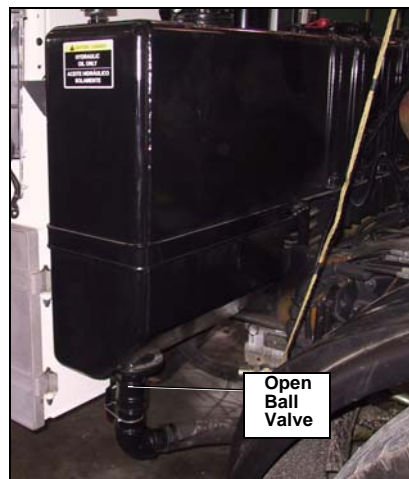
Figure 13. Main hydraulic tank (“saddle” model)
