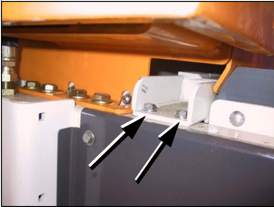
Figure 81. Bolts that retain the beam (two on each side)
