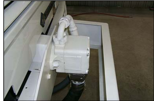
Figure 122. Hydraulic pump on front bumper
