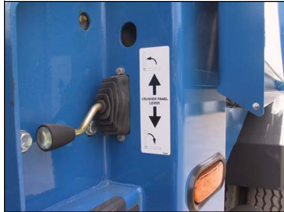
Figure 154. Crusher panel control lever on left-hand side
