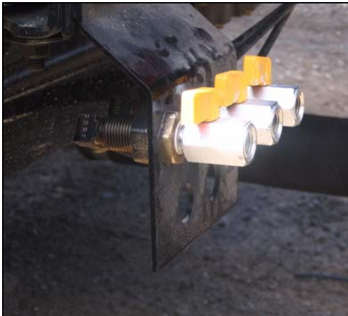
Figure 17. Ball valves with extension hoses
