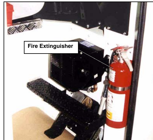
Figure 4. Fire extinguisher location
