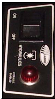
Figure 11. Hydraulic pump switch
