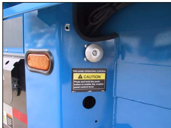
Figure 155. Permission button used to activate the crusher panel control lever on the left-hand side
