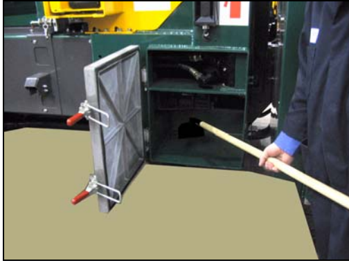
Figure 24. Clean-out trap door
