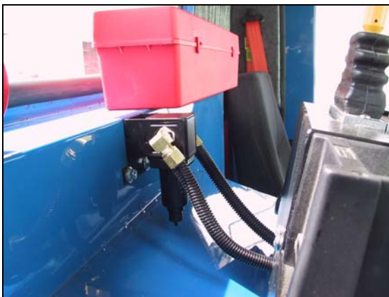
Figure 132. Example of another water trap location
