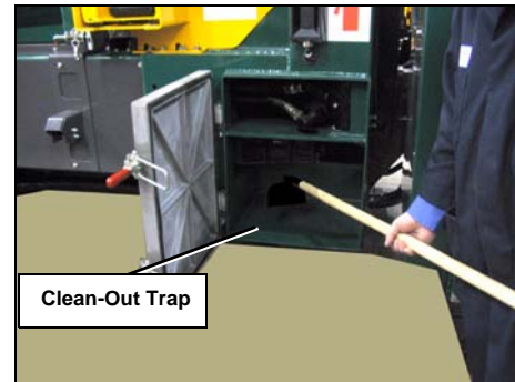
Figure 26. Clean-out trap door
