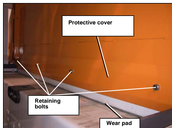
Figure 80. Protective cover (on Helping Hand™-equipped units)
