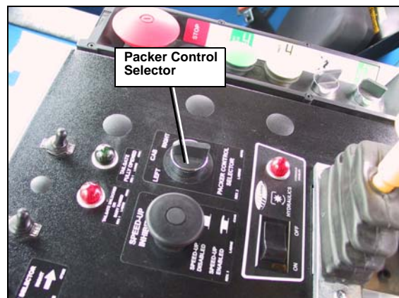
Figure 18. Packer control selector switch
