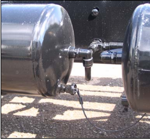
Figure 16. Air tank with steel cable on drain valve
