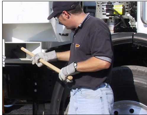
Figure 2-9 Removing debris through the clean-out trap
