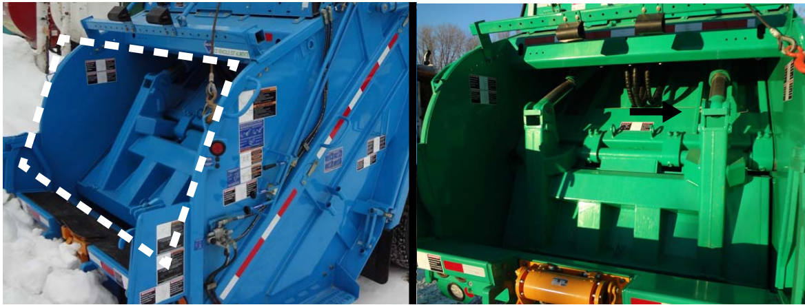
Figure 1-3 Hopper (left); Carrier panel (right)
