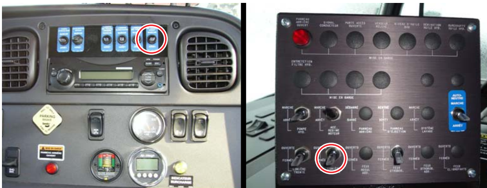
Figure 3-6 FRONT WORK LIGHT switch
