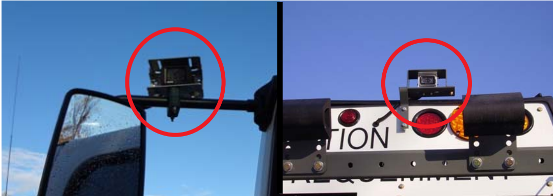
Figure 2-12 Camera on the left-hand side mirror (left), and on the tailgate (right)
