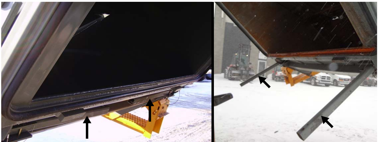
Figure 2-5 Props in stored position (left) and in service position (right)
